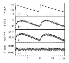
FIG. 3. Time evolution over a day of (a) ESRF beam intensity, (b) tagging-box temperature, (c) CE position and fitted curve [Eq. (5)], and (d)  $\delta = x_{CE} - x_{fit}$ . The error bars on position measurements are directly given by the CE fit.
