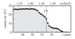
FIG. 2. Si  $\mu$ -strip count spectrum near the CE and the fitting function (see text) vs position *x* and photon energy  $\omega$ . The three edges corresponding to the lines 364, 351, and 333 nm are clearly visible. The CE position  $x_{CE}$  is the location of the central line and is measured with a typical accuracy of 3  $\mu$ m.
