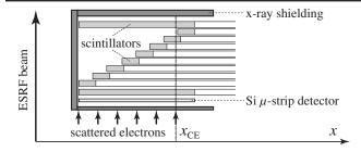
FIG. 1. Schematic drawing of the tagging system.
