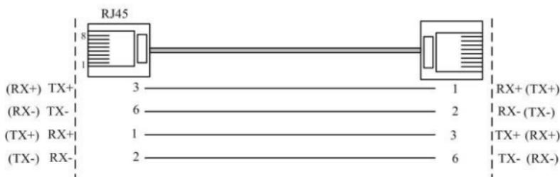
MDI/MDI-X auto connection makes switch easy to use for customers without considering the type of network cable.
