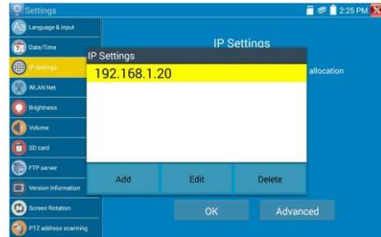
After setting an advanced IP address (refer to the photos above), the unit can test two network segments (192.168.5.0) and (192.168.1.0).
