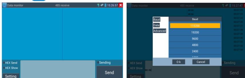
Click “Setting” to choose the baud rate of RS485; it must be the same as the DVR or the Control keyboard .The DVR or Control keyboard send the code to the tester, if it can be read, the protocol will shown on the upper right, like Pelco D, if not, like P:--
