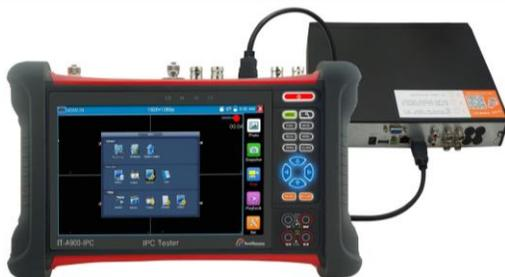
DVR or other device's HDMI out port connect to tester's HDMI in port, the meter will display input image.
