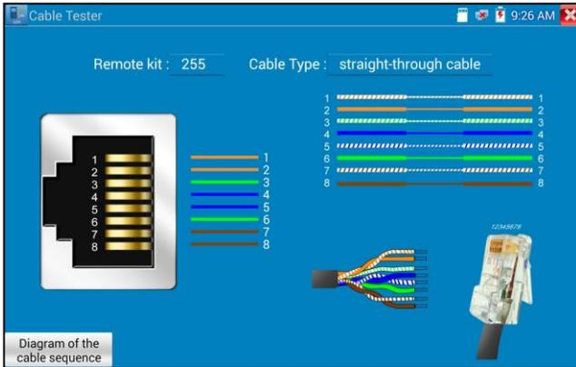
Test LAN cable or telephone cable.
