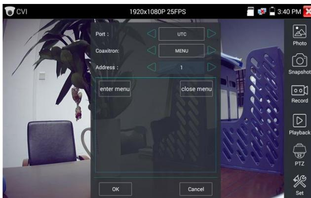
Input calling dome camera menu address code, after finishing the parameter settings, you can press the
