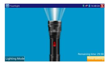
While in the flashlight app, click the red button to turn on the LED lamp. Press it again to turn it off. If you don't press the red button to shut off the lamp and press the button to exit the app, the lamp will stay on. Click the Time Setting button to set a timer that will shut off the lamp.
