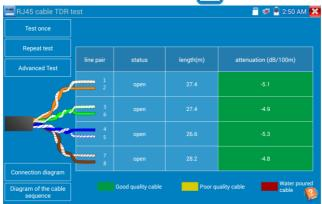
Single test: test cable status, length and attenuation.
