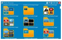
The Media player can browse video and image files. It supports the video formats of MP4, H.264, MPEG4, and MKV. The IP tester recorded files can play directly via the Media player. The Media player will automatically display the video files from the SD card. Click on the desired file to play. Click RETURN to exit.
