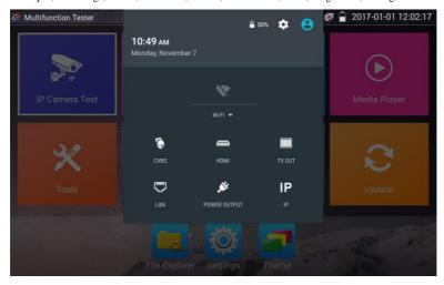
**HDMI:** Click HDMI IN to enter. In HDMI IN mode, it can converter test from analog to digital with dual test window IP & HDMIN or Analog & HDMI in.
