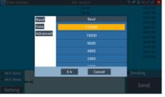
Click "Setting" to choose the baud rate of RS485; it must be the same as the DVR or the Control keyboard. The DVR or Control keyboard send the code to the tester, if it can be read, the protocol will shown on the upper right, like Pelco D, if not, like P:---
