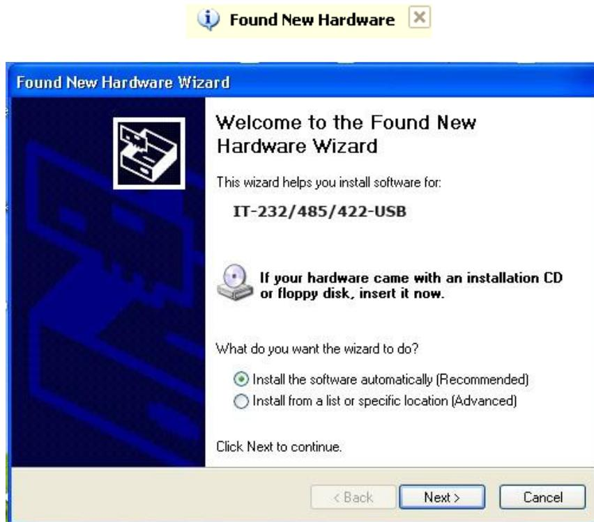
Choice "Install the software automatically (Recommended)", please indicate the driver path to drivers folder in CD's USBxxx file
