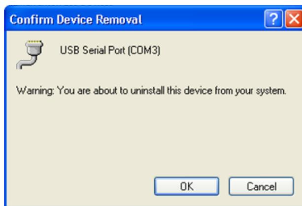
3. In order to install conveniently in next time, please uninstall the memory install, Click "uninstall" and "OK" and finished uninstall, the figure is as follows:
