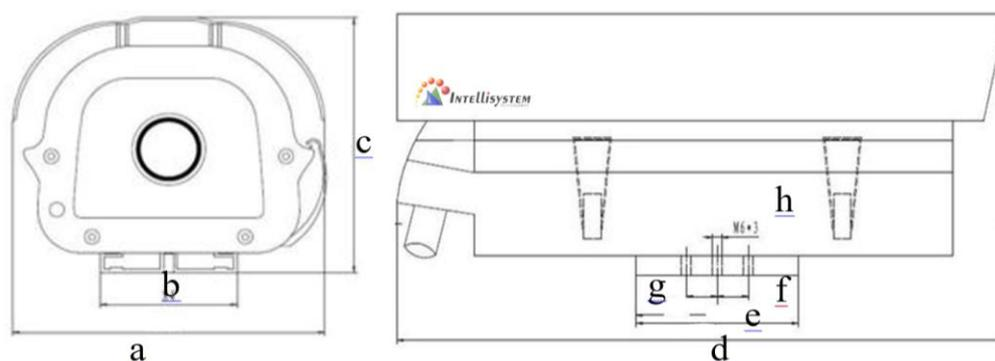
a:172mm b:84mm c:155mm d:480mm e:105mm f:20mm
