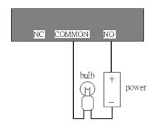
If DI1 in configuration is set as rising to drive DO1 to high that denotes COMMON of DO1 short with NO, then the bulb will light when DI1 signal changes from OV to 12V.
