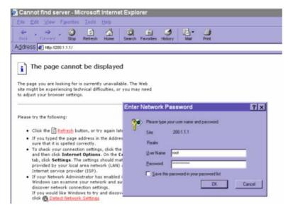
Through direct connection by null modem cable, administrators can connect to "http://200.1.1.1" in the web browser. "200.1.1.1" will be the default IP address of the IT404 Video Server in dial-in connection; "200.1.1.100" will be the given IP address for the user's PC by the IT404 Video Server. The user name and password are the same as what
