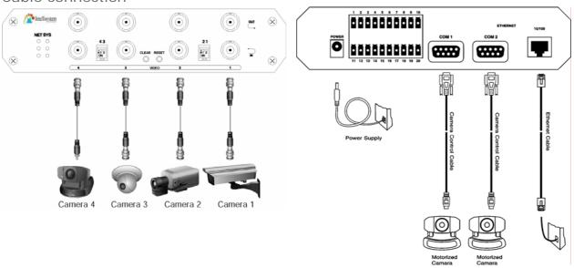
Shut down all the peripheral devices prior to connection. The video BNC, Ethernet cable and power adapter are essential for basic viewing function. If the attached cameras belong to the same motorized model, they can be concatenated to single COM port and will be differed by camera ID set on the cameras. Refer to the related configuration section for detailed description.
