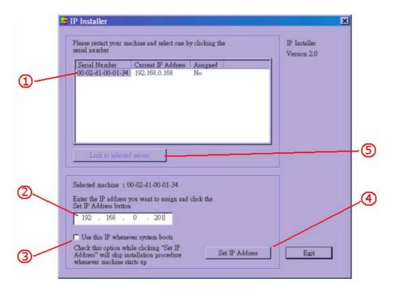
After the POST is done, the IT404 Video Server will try to configure itself by detecting the network environment. If there is DHCP service over the network, the Installer program
