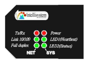
Each time the IT404 Video Server starts up, it will perform power-on-self-test, abbreviated as POST, to examine every hardware module. As soon as the administrator plugs in the power connector both LED's under the power LED will flash one by one until the diagnosis is done. If the result is good, both status LED's will turn off for a while and then follows the pattern below. If any module fails, refer to the Appendix A for the error pattern and
