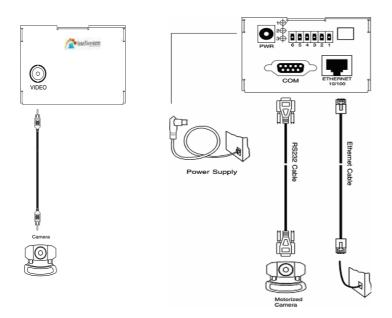
Shut down all the peripheral devices prior to connection. The video BNC, Ethernet cable and power adapter are essential for basic viewing function. If the attached cameras belong to the same motorized model, they can be concatenated to single COM port and will be differed by camera ID set on the cameras. Refer to the related configuration section for detailed description.
