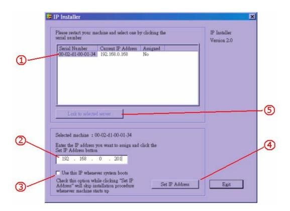
After the POST is done, the IT401 Video Server will try to configure itself by detecting the network environment. If there is DHCP service over the network, the Installer program will catch the given information, then display the serial number and given IP address for each IT401 Video Server as the figure above. To install the IP address, follow the steps.  $\bigcirc$ , 1Click on the entry with the serial number you want to install. If the "Assigned" field
