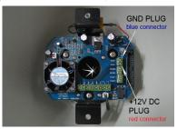
Step 4: Screw on the two side screws, and plug in the power of the dome.
